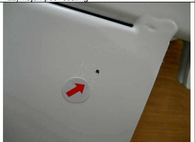
124) Major: poor coating
