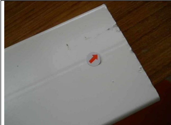
143) Major: poor coating
