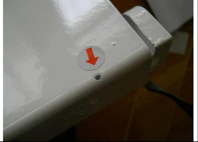
112) Major: poor coating
