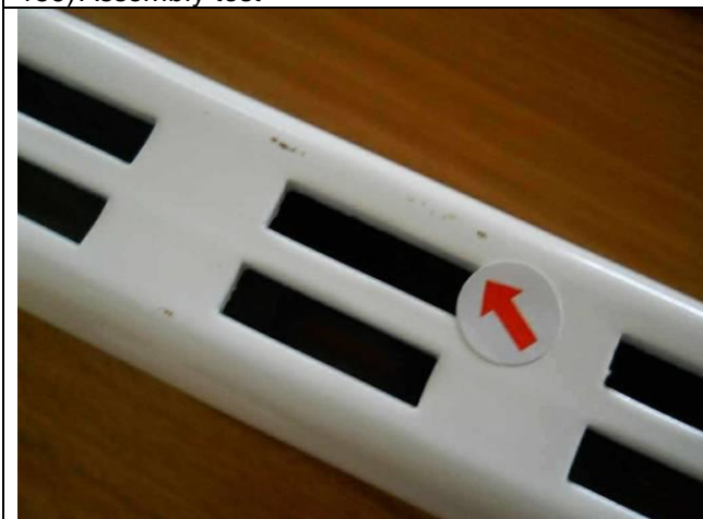
161) Major: poor coating
