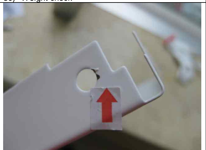
32) Major: poor coating
